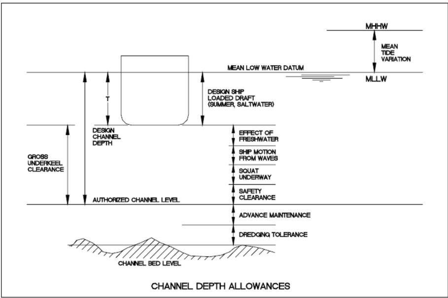
Figure A-1. Channel design depth allowances in deep-draft navigation projects
