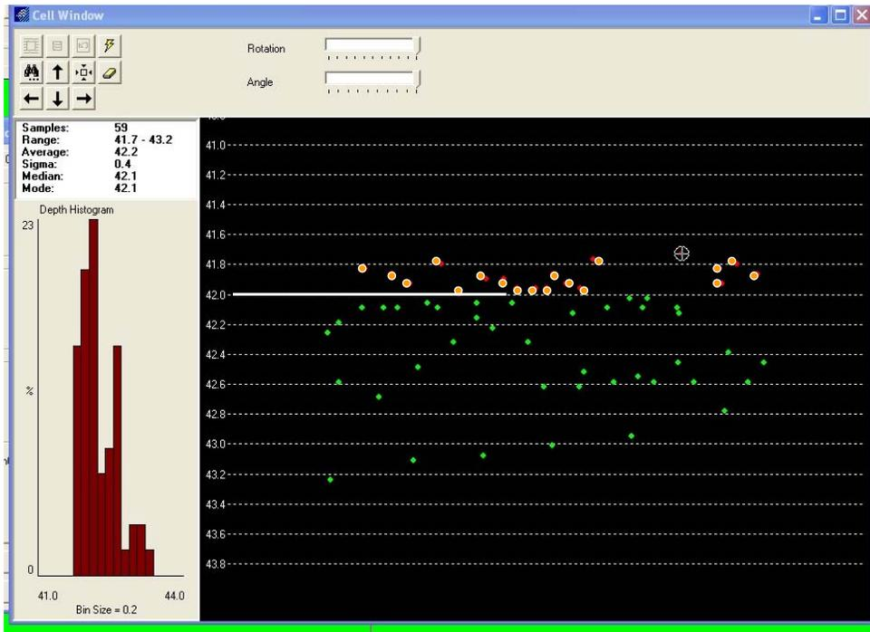
**Figure A-2. Typical dispersion of 59 individual multibeam depths observed in a 3 ft x3 ft cell—multiple passes over a suspected strike in a rock-cut turning basin. Depths above the required 42-ft grade are highlighted. Miami Harbor—Jacksonville District (2006)**
