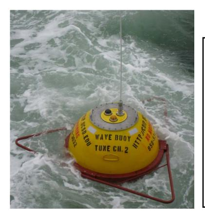
Buoys measure wave height, wave direction, wave period and sea surface temperature. The data are broadcast on the NWS Marine Weather Channel, and are also disseminated in near real-time on the web at <a href="http://cdip.ucsd.edu">http://cdip.ucsd.edu</a> (click on RECENT).
