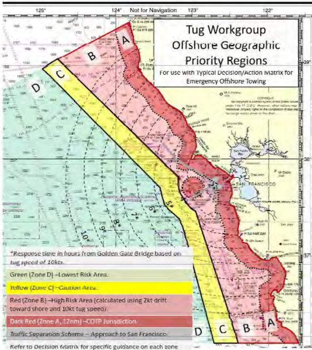
Figure 1: Safety Risk Associated with Vessel Position Offshore
