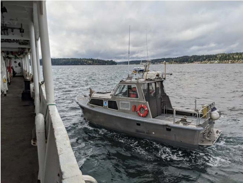
Survey launch that will be doing the majority of survey work, especially in shallow waters and nearshore, etc.
